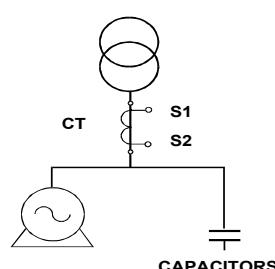
The current transformer , CT, must be located so that it measures the whole load current plus the correction capacitors
